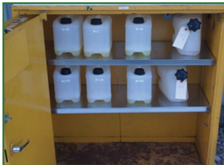
Dr. Greg Davis, an ethanol researcher at Kettering University, has performed numerous small-engine phase separation studies including this storage test.
